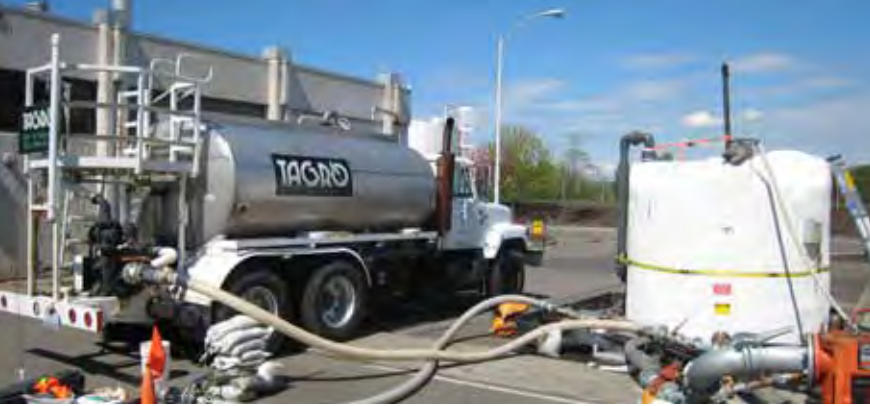
PILOT TESTING AT THE TACOMA CENTRAL TREATMENT PLANT OF HAULED LIQUID WASTE FOR CO-DIGESTION
